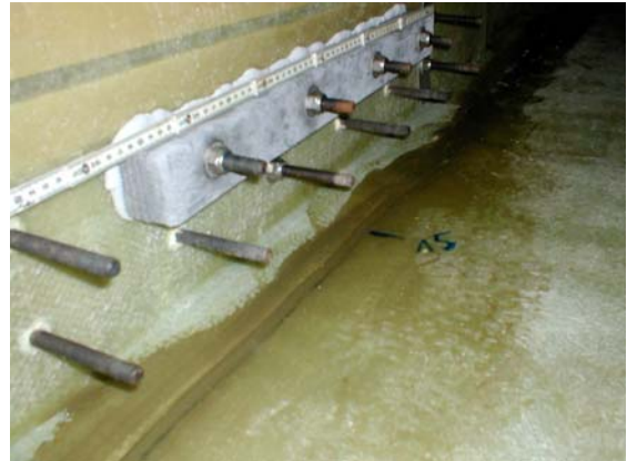
Fig. 8: Threaded rods for balancing weights in a rotor blade
