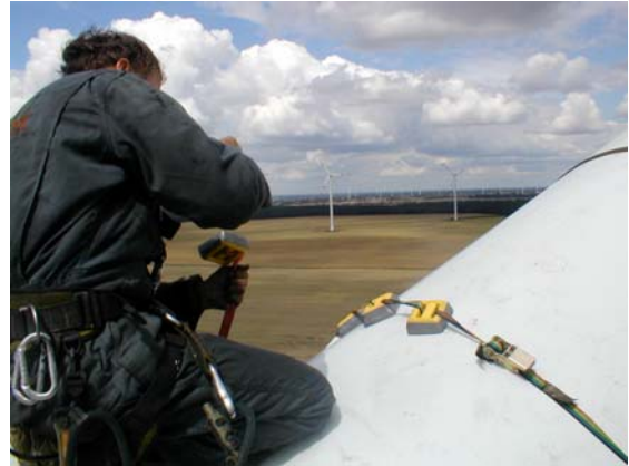
Fig. 7: Attachment of test weights at the blade root
