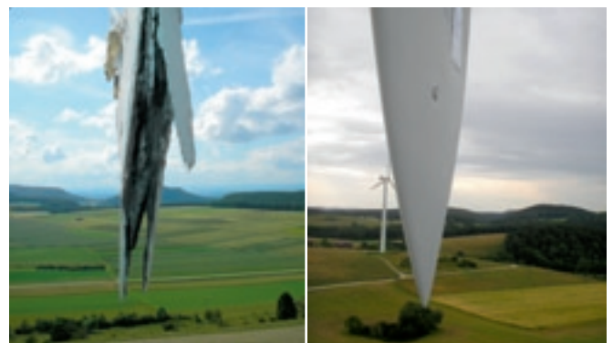
Damaged blade tip before repair (left) and after repair (right)
